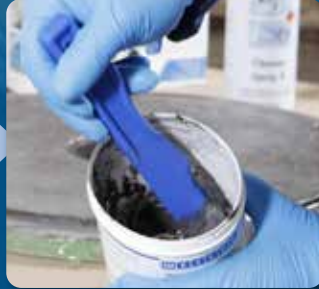
Mix resin and hardener thoroughly and bubble-free
