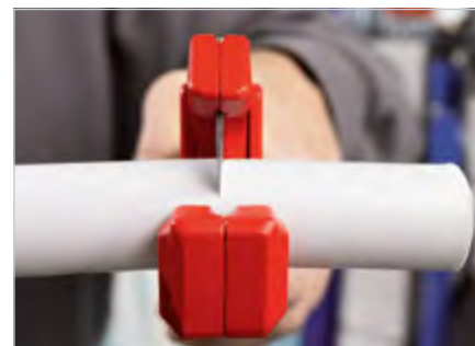
Enables a straight and right-angled cut
