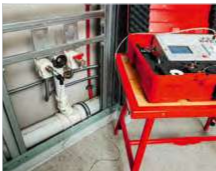
High pressure sensor already included in the set for testing water pipes – also with test medium water
