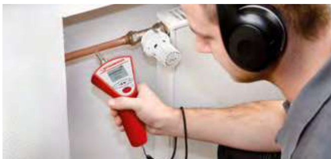
Acoustic leak detection of heating installations
