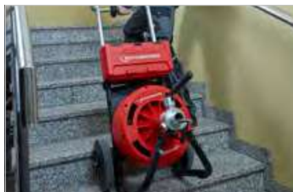
Easy transport due to stair capable chassis
