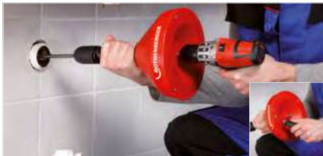
Electrical operation with cordless drill
